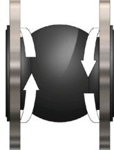
The twisting of one end of the expansion joint with respect to the other end about its longitudinal axis.
