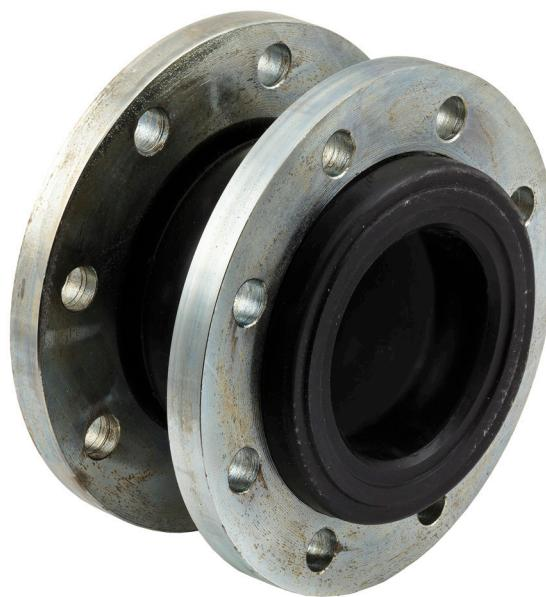
Rubber expansion joints are designed to alleviate piping stress, absorb pipe misalignment, compression and extension, noise and vibration, in a relatively short space. Standard stock items are the single arch and the twin-sphere joints. The spherical shape arch of the connector and excellent original structural design contribute to the great success of the joint.
