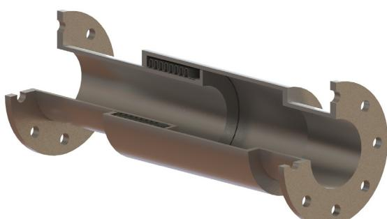
When the pipe expands, it compresses the expansion joint but extends the bellows. The bellows element remains stable due to the external pressure acting upon it.
