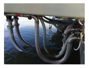
The specialist hose design can also be used to contain hazardous medium in the event of a rupture. The outer hose will capture any medium that leaks from the inner hose preventing any safety or environmental issues. Sensors can be installed on the ports of the outer hoses to analyse any changes in pressure or gas detection.
