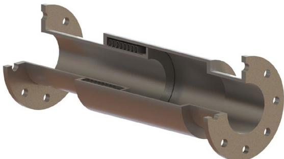
When the pipe expands, it compresses the expansion joint but extends the bellows. The bellows element remains stable due to the external pressure acting upon it.
