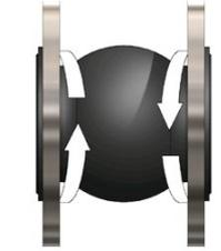
The twisting of one end of the expansion joint with respect to the other end about its longitudinal axis.
