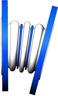
“Maximum Angular Deflection” may be called angular rotation. It is based on installation with no axial travel or lateral offset.
