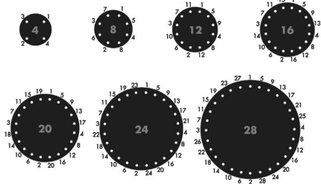
Tighten bolts in stages by alternating around the flange. Use recommended torque values above to achieve a good seal. Never tighten an expansion joint to the point that there is metal-to-metal contact between the expansion joint flange and the mating flange.
