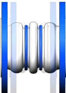
“Maximum Axial Travel” may be called longitudinal movement or axial compression and extension. It is based on installation with no misalignment or angular deflection.
