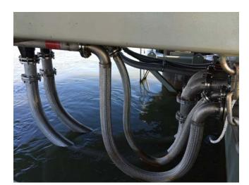
The specialist hose design can also be used to contain hazardous medium in the event of a rupture. The outer hose will capture any medium that leaks from the inner hose preventing any safety or environmental issues. Sensors can be installed on the ports of the outer hoses to analyse any changes in pressure or gas detection.
